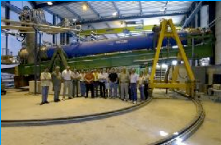
CAST (LHC dipole 9.3 m, 9T)
