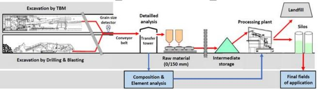
Graphic representation of underlying forecast reliability and associated recovery and landfill classes of a tunneling project in phase A of the main investigations (ÖBV 2015)
