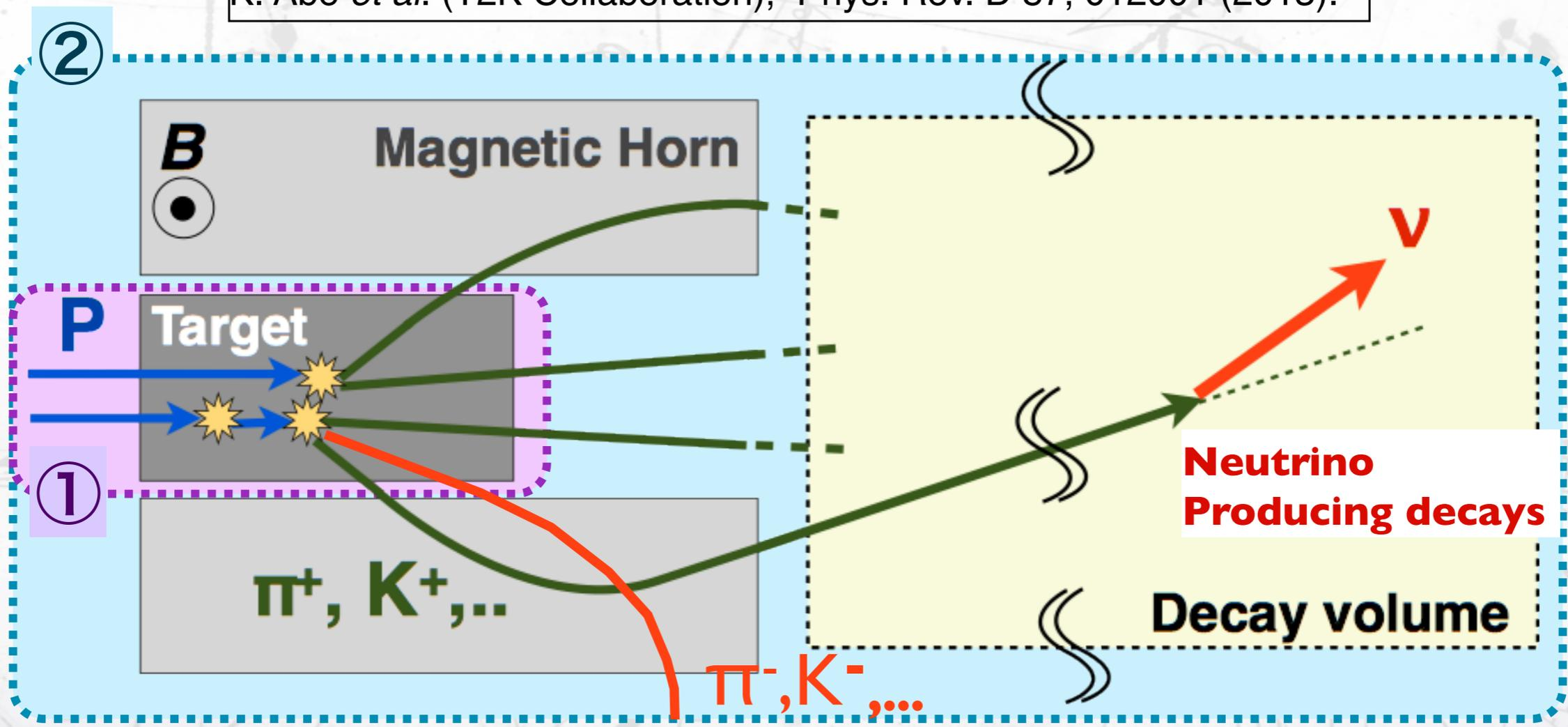
To make antineutrinos we simply reverse the B field changing the horn current pulse polarity.
