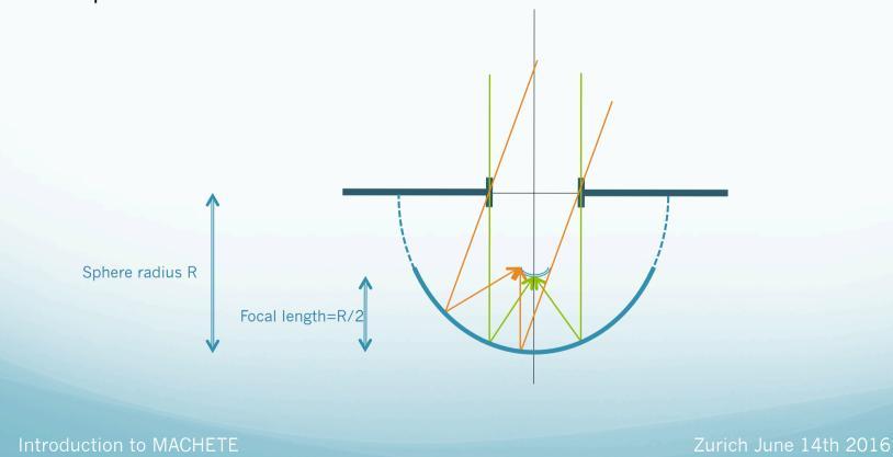
STEP 4. Add the Schmidt **corrector plate** at the stop. That eliminates spherical aberrations.
