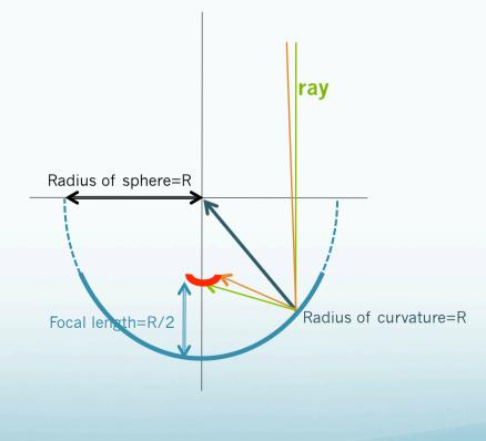
STEP 3. For a spherical mirror as rays hit further and further away from optical axis they get more a more defocused.
