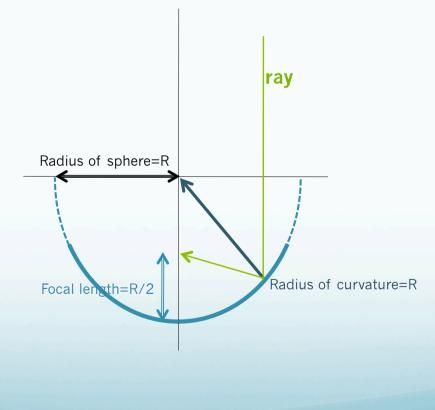
STEP 2. Make the **focal plane spherical**, with center at center of mirror. All incident directions become equivalent.
