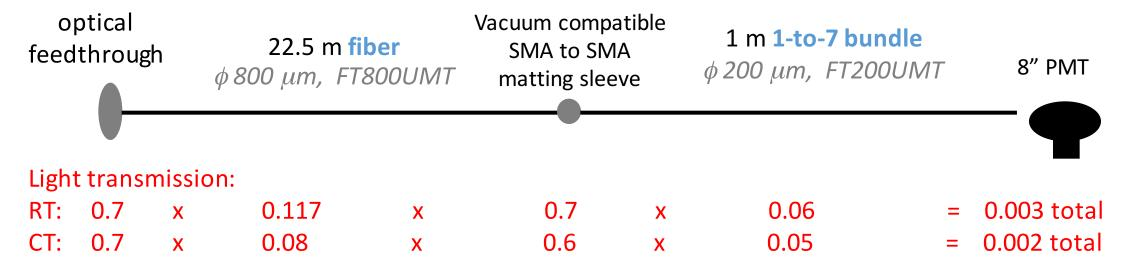
Assuming homogeneous light at SMA flange feedthrough Measured in different steps, need to measure everything together
