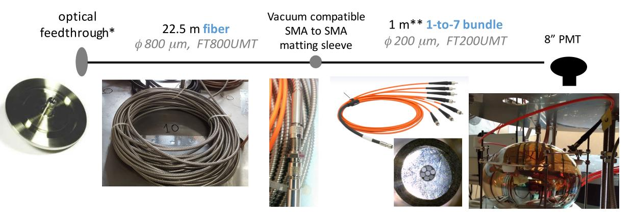
\*Final design 3 feedthroughs per flange
