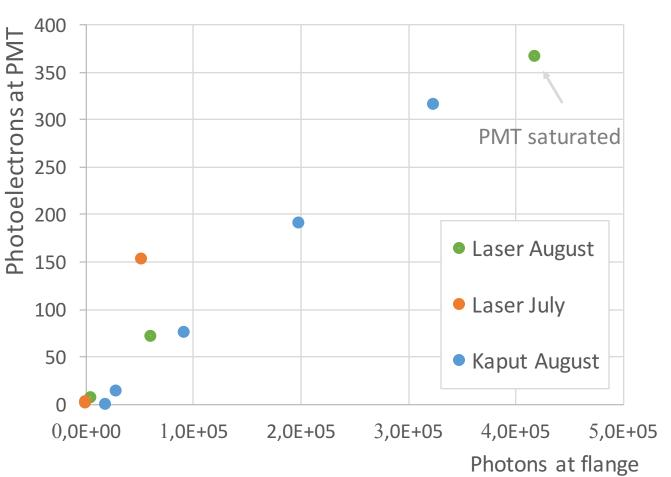
NPE at PMT vs NP at flange
