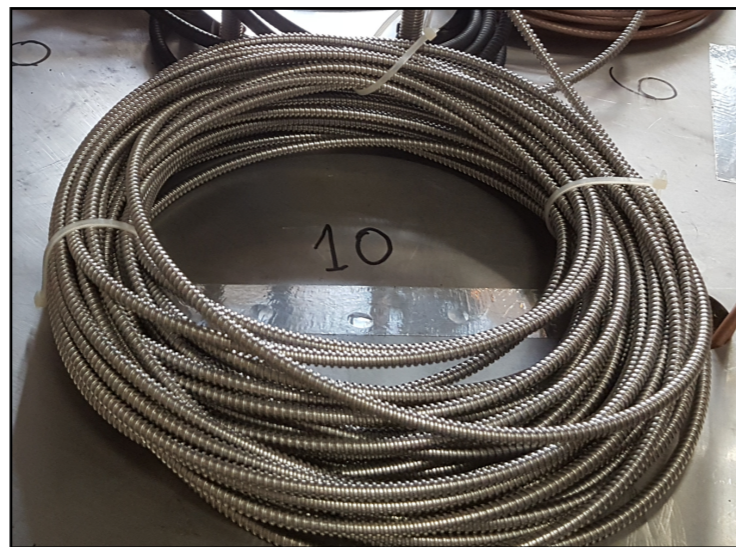
[x7] Fibers (Thorlabs): FT800UMT, \varnothing 800\mu\text{m} , L 22.5m, SMA connectors
