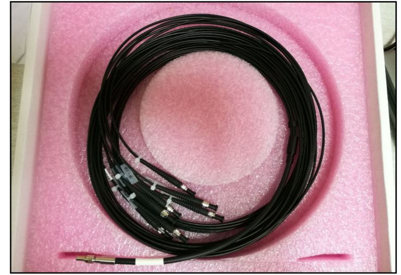
[x7] 1-to-7 fiber bundles (Thorlabs): FT200UMT, \varnothing 200\mu\text{m} , L 3m, SMA connectors
