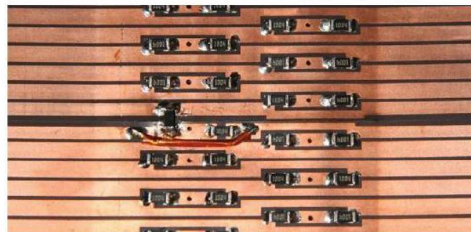
Figure 5.13: Resistor chain in the field cage at the central connection between the half boards
