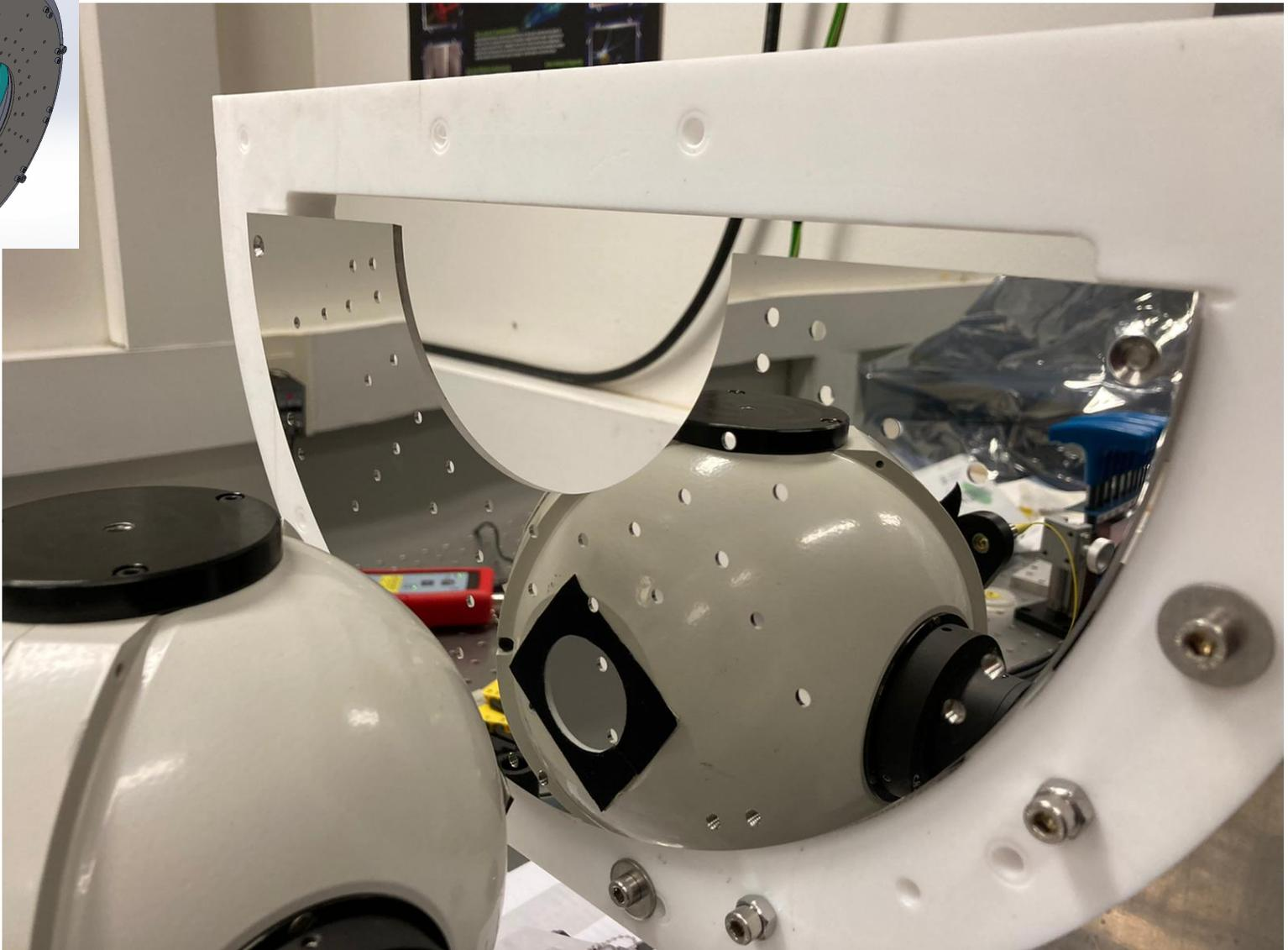
**AISI 304L stainless steel polished ½ baffle being tested for TIS**
