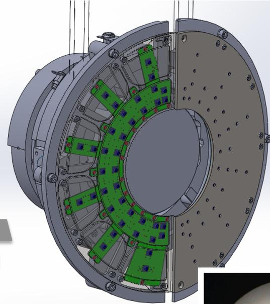
$\rightarrow$  Full R&D performed to achieve the level of precision required in RoC in the baffle edges  $\rightarrow$  Drilling + lapping using inserts
