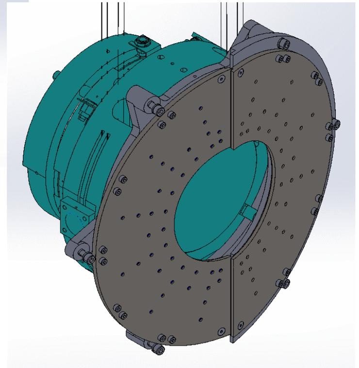
Instrumented baffles with photo-sensors surrounding mirror
